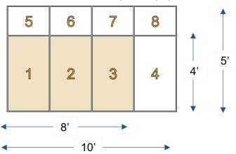
Our CNC machine features 8 suction zones meticulously designed to handle 5'x10', 4'x8', 4'x10' and 5'x8' sheets, as well as small offcuts. Each of these zones can be controlled individually from the operator control station with just the click of a button. The innovative V-groove table design ensures that vacuum suction power is evenly distributed across each zone, optimizing performance and efficiency.
