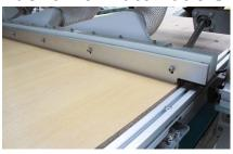
A CNC pusher unloader becomes essential when you're focused on maximizing efficiency and streamlining workflow in high-volume production settings. This feature automates the unloading process by pushing finished materials off the table, readying the machine for the next cycle without requiring manual intervention. Our pusher comes with air blowing nozzles and dust collection chute to eliminate any dust from working table. (Must be purchased if planning to add unloading conveyor belt later)
