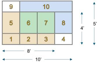
Our CNC machine features 10 suction zones meticulously designed to handle 5'x10', 4'x8', 4'x10' and 5'x8' sheets, as well as small offcuts. Each of these zones can be controlled individually from the operator control station with just the click of a button. The innovative V-groove table design ensures that vacuum suction power is evenly distributed across each zone, optimizing performance and efficiency.
