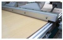
A CNC pusher unloader becomes essential when you're focused on maximizing efficiency and streamlining workflow in high-volume production settings. This feature automates the unloading process by pushing finished materials off the table, readying the machine for the next cycle without requiring manual intervention. Our pusher comes with air blowing nozzles and dust collection chute to eliminate any dust from working table.
