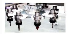
A 16-position automatic tool change carousel is a game-changer for productivity and versatility. With 16 slots, operators can load a diverse range of tools in advance, which means fewer interruptions and faster transitions between operations. This setup minimizes downtime and ensures that our CNC can handle complex jobs with multiple tools seamlessly, boosting efficiency and cutting down on manual tool changes. This flexibility is a major asset in high-paced production environments.
