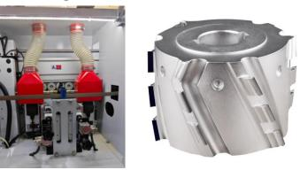
Pre-milling with two motors and 45 mm diamond cutters ensures precise, smooth panel edges by removing imperfections and maintaining symmetry. Diamond knives stay sharp longer, handle thicker panels effectively, and improve edge-banding quality, making the process ideal for high-gloss or solid wood applications.
