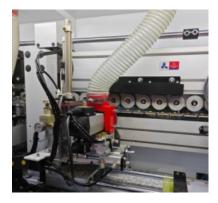
Having corner rounding in an edgebander is highly beneficial for achieving perfect rounded corners, especially for edges that cannot be corrected after end trimming, such as rounded, duckbill, or rightangle corners. This feature allows for precise modifications, ensuring a flawless finish.
