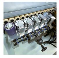
Our edgebander is equipped with two pneumatic pressure rollers designed for exceptional edge-banding performance. Each roller features its own independent pressure control valve, ensuring precise adjustment for various materials and thicknesses. Additionally, every roller is fitted with a knife for self cleaning, guaranteeing superior quality.
