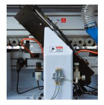
Our edgebander is equipped with two independent high-frequency motors that precisely trim the remaining material at the front and back ends, delivering a clean and smooth finish. The motors operate on a precise linear guide rail system, ensuring seamless movement and exceptional cutting accuracy. An automatic rail lubrication system enhances durability and performance, while a cylinder with a pressurereducing valve provides reliable and consistent operation.
