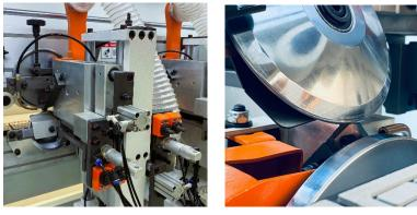
Manual control mode, with a small profile wheel driven by a linear guide rail, ensures precise positioning. No power scraping required; the tool pattern is removed after trimming, creating a straight and full arc. Suitable for PVC/ABS edgebanding up to 3mm with scraped edges
